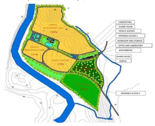
Picture 1 – Layout of South Tangerang Waste to Energy
