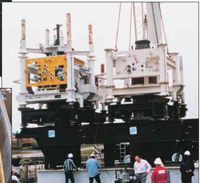
Fit-and-function test of a Subsea Tree on a DRIL-QUIP Modular Drilling and Production Template System
